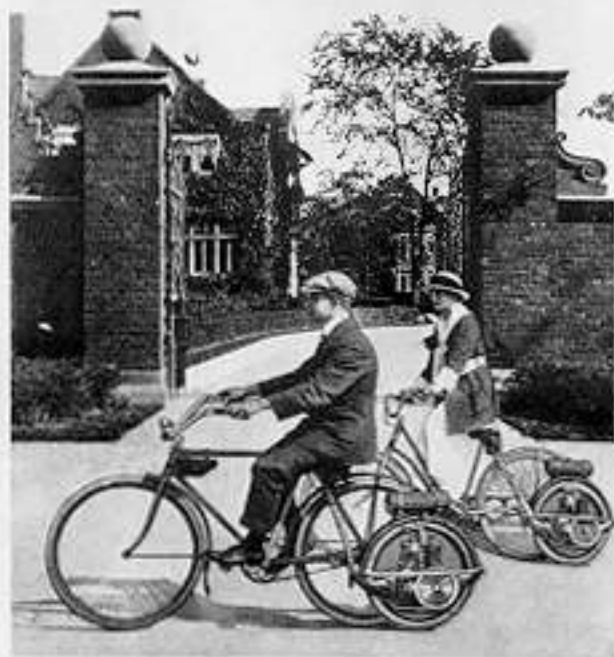
Two bicycles equipped with Smith Motor Wheels, around 1917-18. Photo from the Automotive History Collection, Detroit Public Library.
