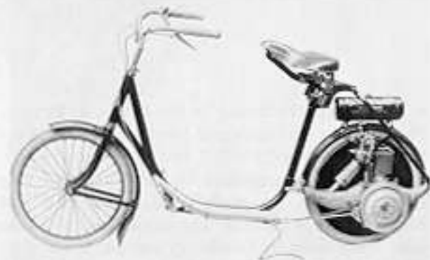
In this photograph, a Motor Wheel powers a Briggs & Stratton Scooter.
