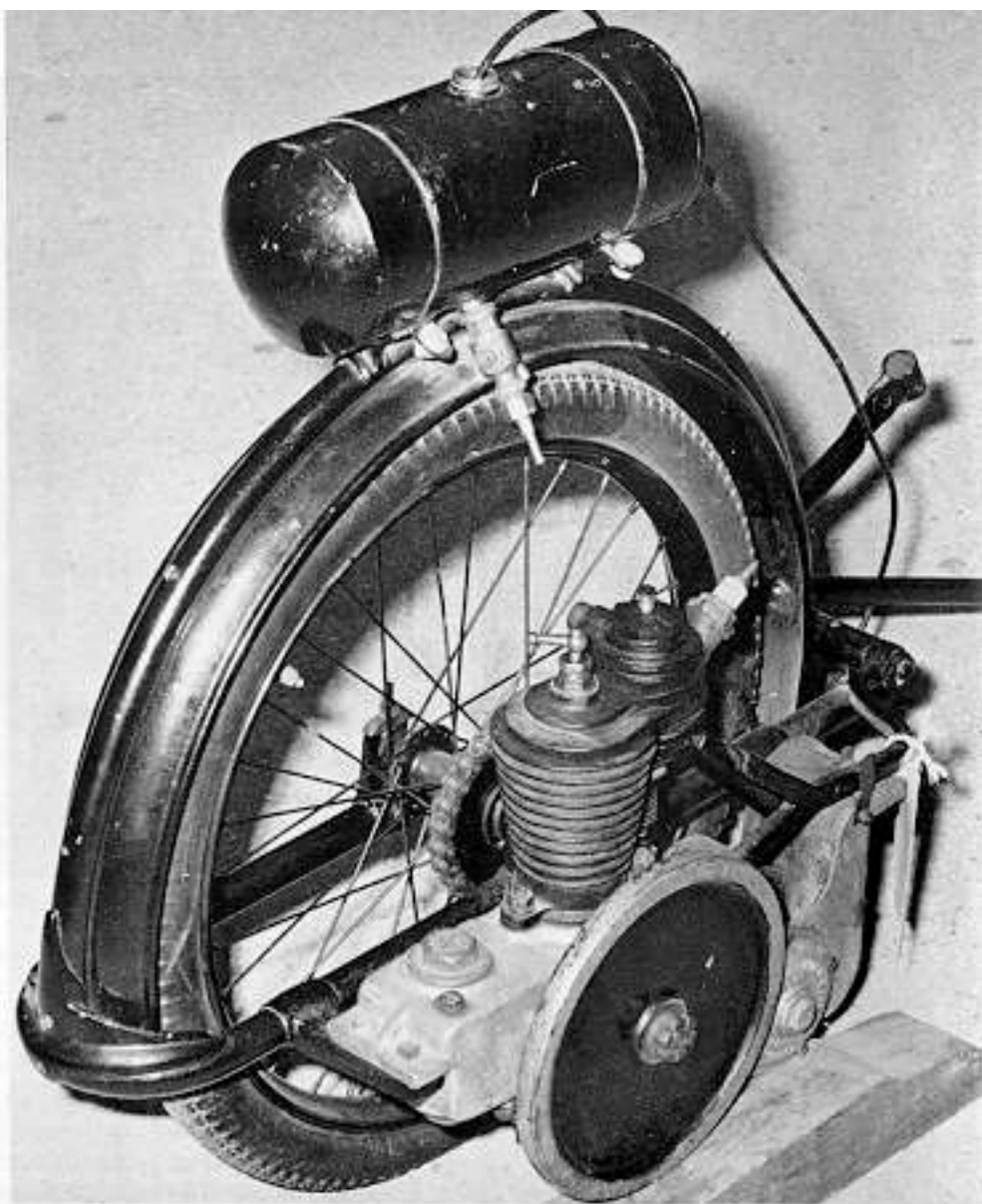
1912 Wall Auto Wheel with chain drive and wire wheel. Photo from the Montagu Motor Museum collection in England.
